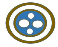
Individual Steel Pipes bundled together inside a carrier pipe
