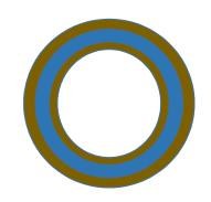
Steel Pipe inside another steel pipe with Polyurethane Fam in between
