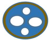
Bundle of steel pipes inside a carrier pipe with insulation foam in between
